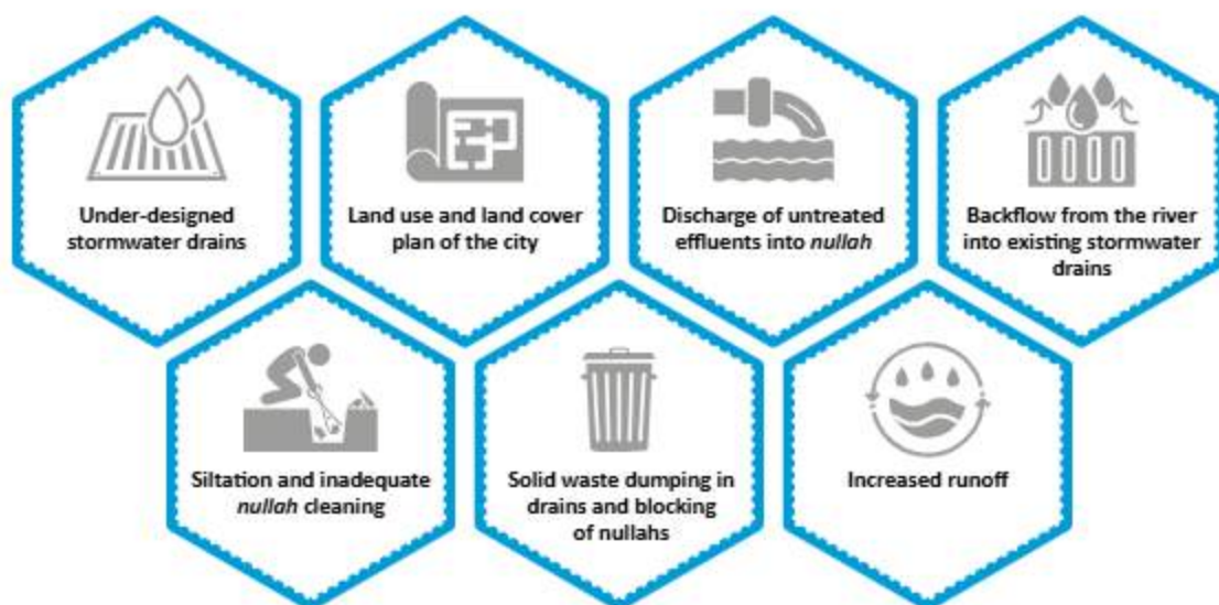
Figure 4: Emerging pressures revealed on the stormwater drainage network within NMC
