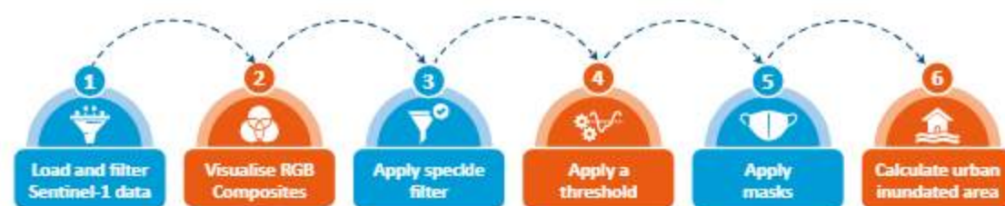
Figure 6: Flood inundation mapping carried out through a series of systematic steps
